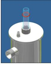
Screw again the sleeve bolts and insert the lamp holder spring into the sleeve:
