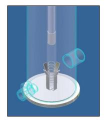
Insert the o-ring  $\emptyset$  23x4 into the quartz sleeve:
