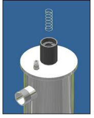
In case of LCD PLUS UV system: Mount the o-ring (3043 type) on the probe holder and screw this one on the  $\emptyset$  <sup>1</sup>/<sub>4</sub>" bush welded in the middle part of the UV chamber. Finally, connect the pertinent electrical cable:
